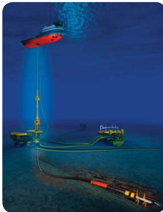
FMC Technologies is currently using Riserless Light Well Intervention in the North Sea on wellheads as deep as 550 meters (1,815 feet). It plans to extend the range to one kilometer (more than a half mile) by 2007.
